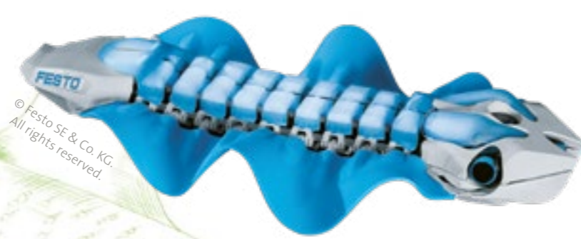
This small underwater robot glides through the water like a cuttlefish. Two servomotors drive the silicone fins on its side.
