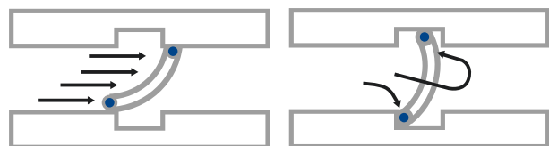
Inside sealing – groove in housing
